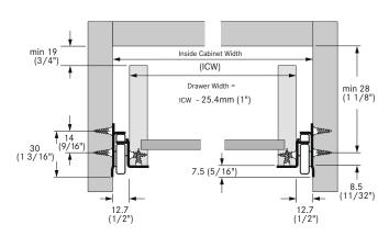
Manufacturing often is accompanied by tolerance problems. To avoid this situation, Grass slides are designed to eliminate side movement of the drawer. After installation, the right drawer member blends perfectly with the right cabinet member for guidance: the left side allows for cutting tolerance of the drawer and the cabinet components.
