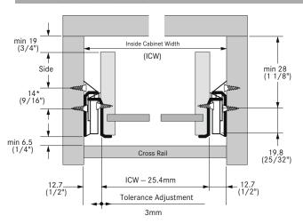
Manufacturing often is accompanied by tolerance problems. To avoid this situation, Grass slides are designed to eliminate side movement of the drawer. After installation, the right drawer member blends perfectly with the right cabinet member for guidance: the left side allows for cutting tolerance of the drawer and the cabinet components.
